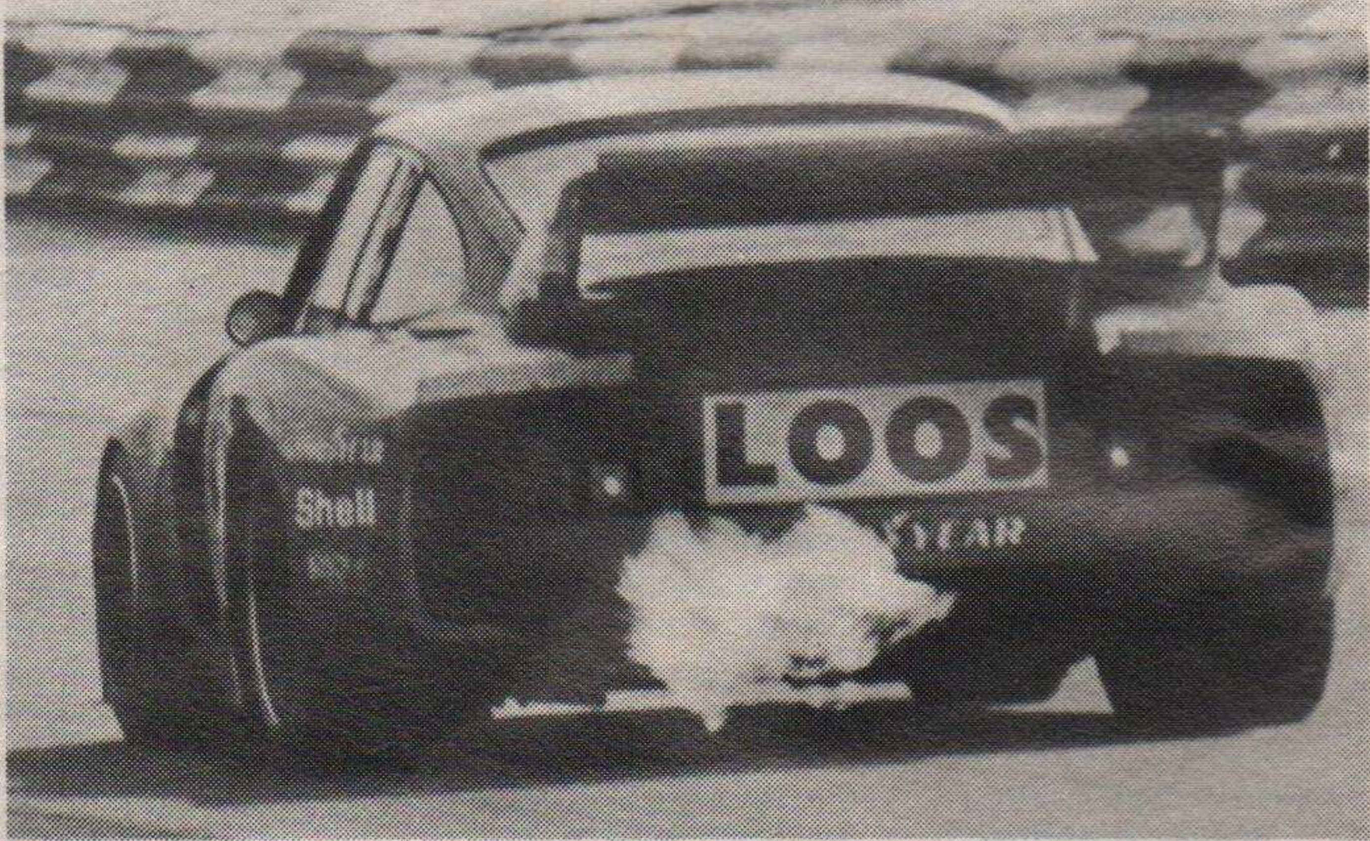
Typical "flame out" on the over-run of a turbocharged Porsche 935.
